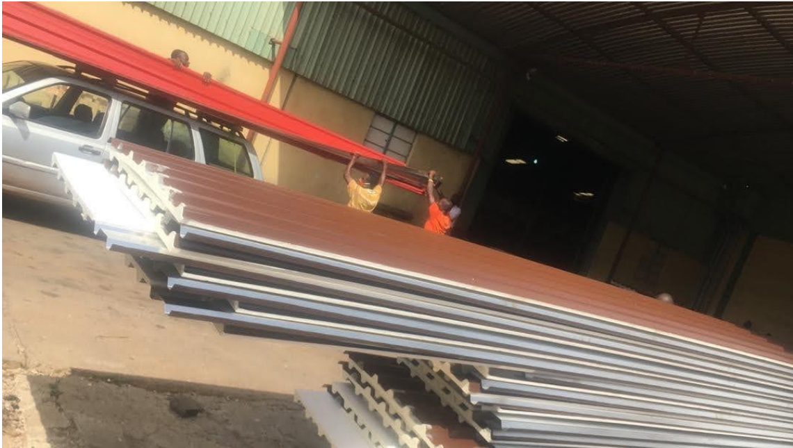
5 – POLYURETHANE FOAM ALUMINIUM ROOFING SHEET, IKEJA GRA.
